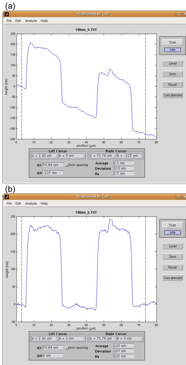
Figure 11: Leveling data. (a) The data starts out slanted, so the left and right cursors are placed to determine the leveling points. (b) Once the *Level* button is clicked, the data shifts according to the left and right cursors and results in better leveled data.
