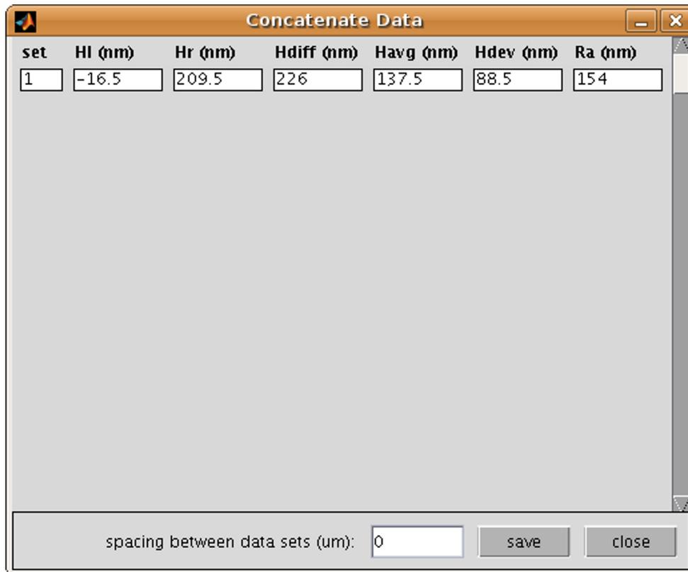
Figure 12: The concatenate data menu the first time it is called. It loads the following values determined by the position of the left and right cursors: the data set number (set), the left cursor height measurement (Hl), the right cursor height measurement (Hr), the height difference between the cursors (Hdiff), the average height between the cursors (Havg), the deviation of the height between the cursors (Hdev), and the surface roughness between the cursors (Ra).
