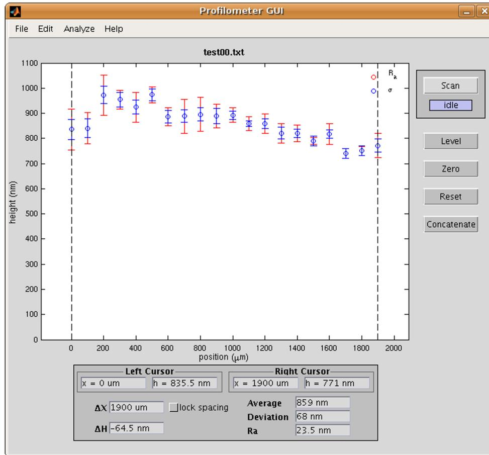
Figure 15: Concatenated data plotted in the program window. The data shown here represents the average height for several features with blue error bars indicating deviation and red error bars indicating surface roughness.
