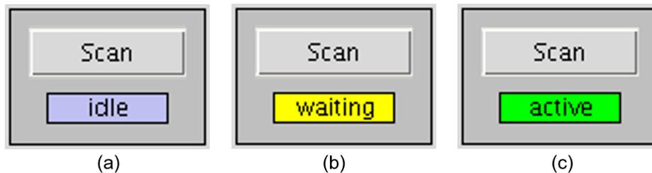
Figure 2: Values that the scan field can assume. (a) When status is set to *idle*, the program is not checking for data from the profilometer. (b) When the status is set to *waiting*, the program is actively watching for data to be sent to the serial port from the profilometer. (c) When the status reads *active*, data is currently being transferred.
