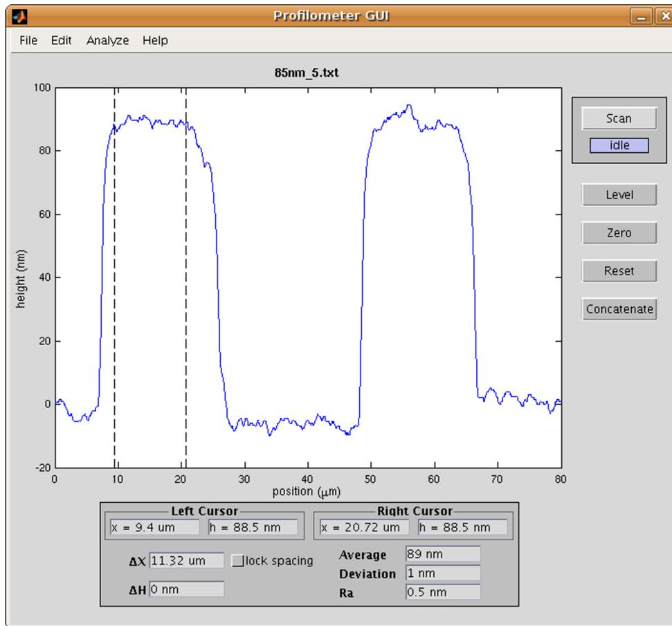
Figure 10: The left and right cursors are used over a somewhat flat segment of this feature to highlight the height average, deviation, and the surface roughness. In this case, the average is displayed as 89 nm with a deviation of 1 nm, and the surface roughness is shown as 0.5 nm.
