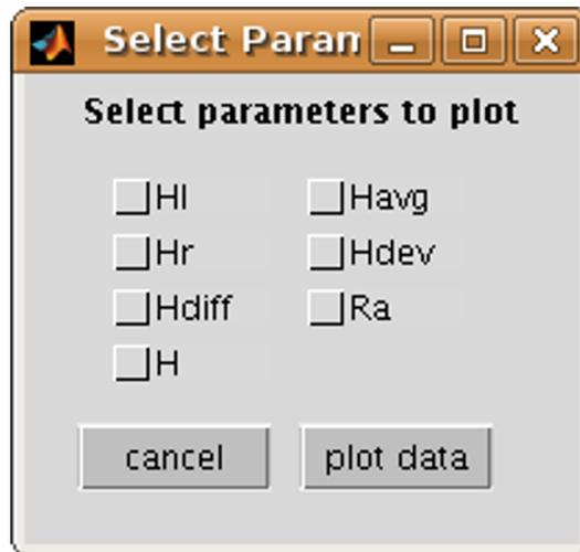
Figure 14: When loading a concatenated data set, this menu allows you to select what to plot. You can plot either the left cursor height (Hl), the right cursor height (Hr), the difference in height between the cursors (Hdiff), all of the data points between the cursors (H), or any combination of the average height (Havg), the deviation (Hdev), and the surface roughness (Ra).
