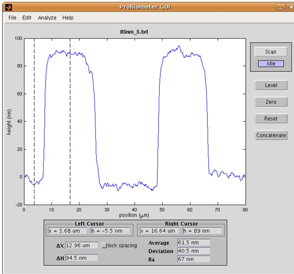
Figure 9: The usefulness of using the left and right cursors to measure the step change from one feature to another. The left and right bars are shown placed on the feature on the left of the plot. The displayed height different,  $\Delta H$ , is 94.5 nm.
