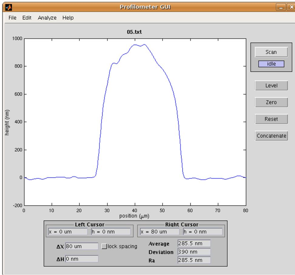
Figure 5: A loaded file plotted in the program window. The title in this example, *05.txt*, indicates that this is data that has been saved after being read in from the profilometer or that it was loaded from an existing text file.
