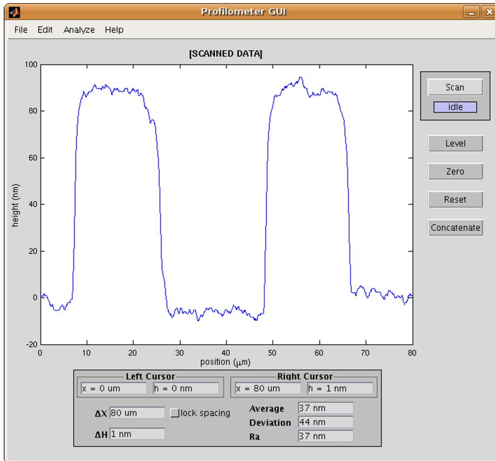
Figure 3: Once data is retrieved from the profilometer through the serial port, the resulting scan is plotted in the program window. The title *[SCANNED DATA]* indicates that the current plot was scanned directly from the profilometer and has not been saved.
